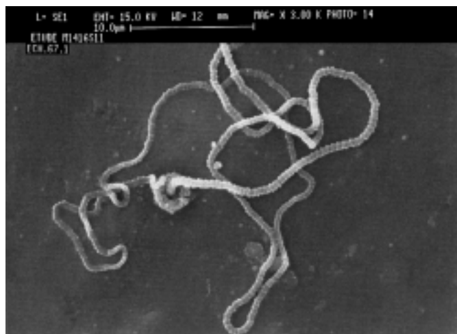
Figure 4. SEM image of PPy/CIO 4 wires grown from a PEA grafted carbon electrode.
